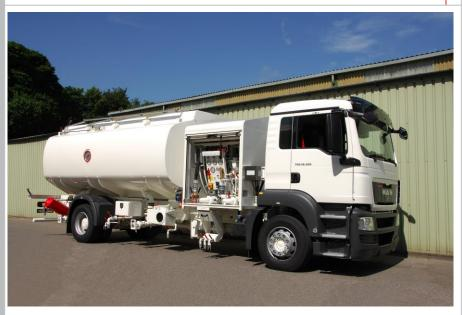
A 20,000L useable capacity rigid refueller mounted on either a 4x2 Scania chassis. The refueller is equipped with 1 x underwing and 1 x overwing hose, single meter and filter water separator or an optional filter monitor. Options include a weatherproof cabinet. The refueller conforms to latest European Standards EN12312-5 and JIG1 Issue 12 requirements.
